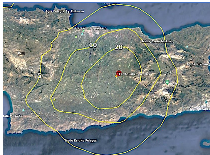
Figure 2. Shakemap of the M6.0 earthquake in Arkalochori, Crete, in terms of maximum ground acceleration (iso-contours of [%g], g: acceleration of gravity). Triangles indicate the accelerometer stations recorded the ground shaking( http://shakemaps.itsak.gr ).
