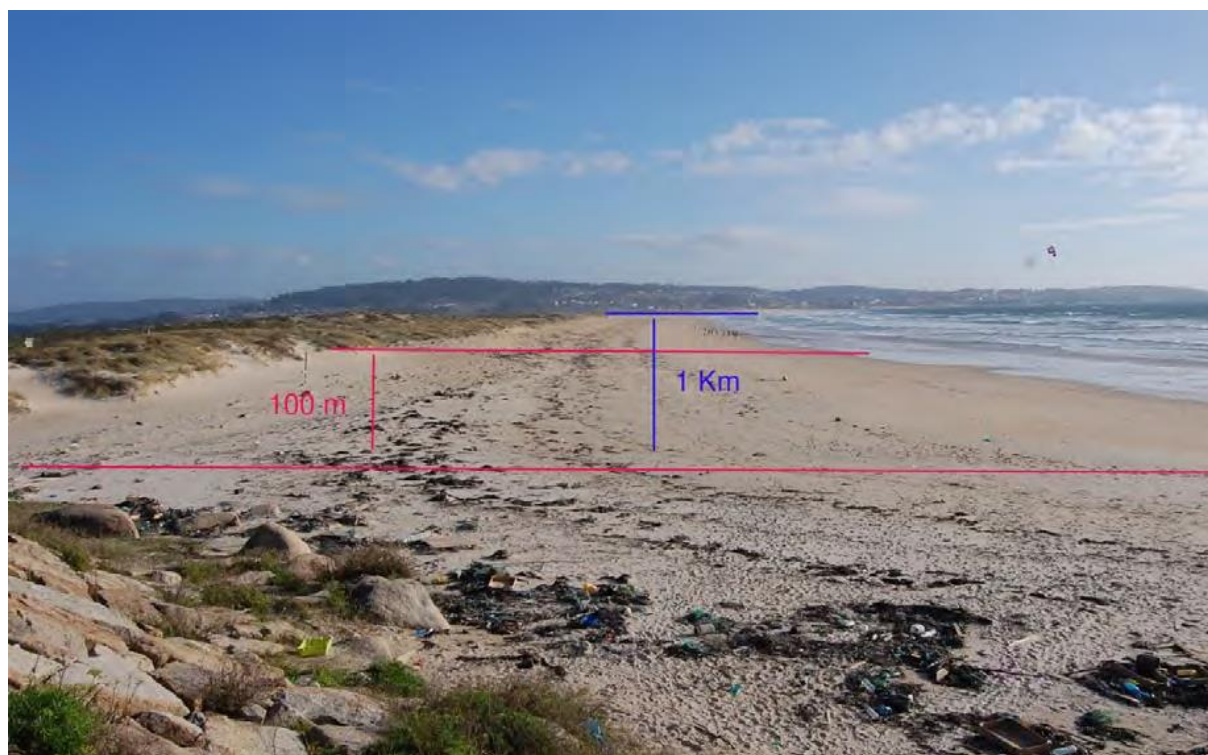
Fig. 10 Schematic diagram for monitoring of sea beaches according to the Guideline for monitoring marine litter on the beaches in the OSPAR maritime area
