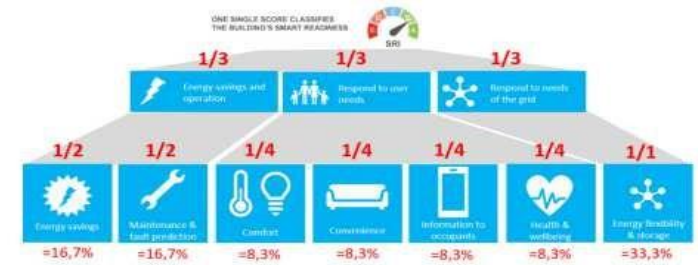
Figure 13 – Aggregation of impact scores to three key functionalities or to a single score
