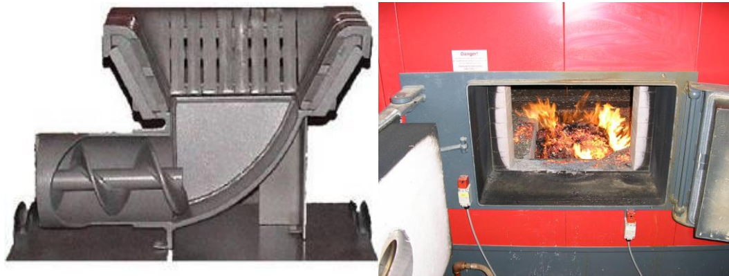
Underfed Hearth – Chip Fed in from side via fuel augers
