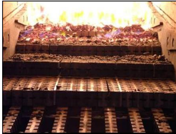
Mechanically Driven Step Grate combustion chamber with wetter wood chip moved along the combustion chamber as it dries
