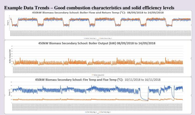
Datasets show good combustion characteristics during varying heat loads.
