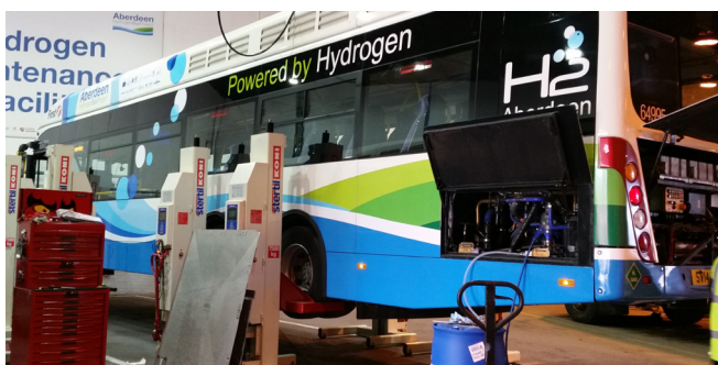
Figure 21: VanHool Bus in for Schedule Maintenance at the Aberdeen Hydrogen Maintenance Facility in Kittybrewster Depot
