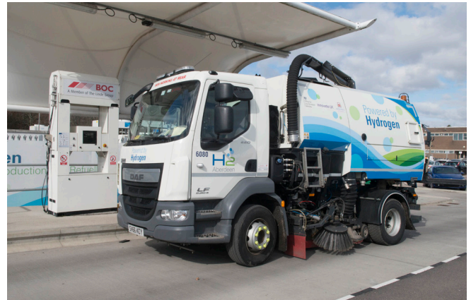
Figure 13: Road Sweeper Retrofit DAF LF 220 FA Johnson Sweeper 16 Tonne
