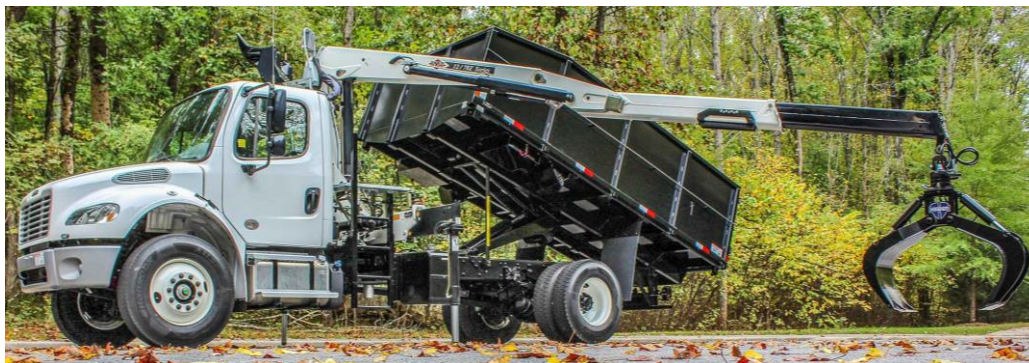
Figure 21: Dump truck, hydraulic arm and grab head. ( https://www.customtruck.com/ )
