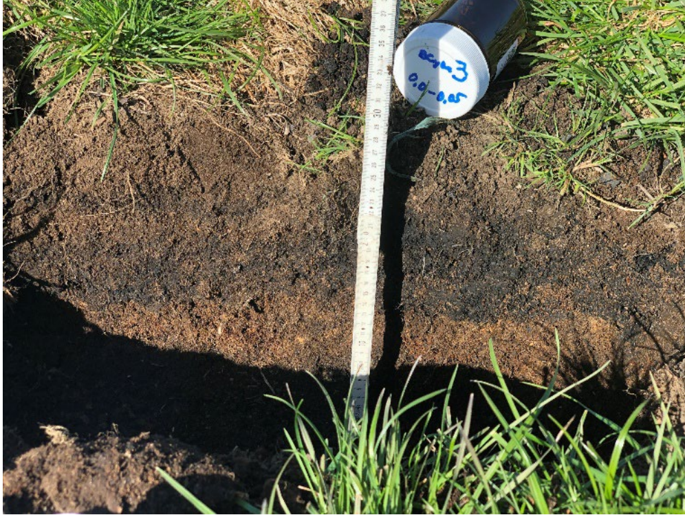
Figure 24. The dispersion of TOC indicating biochar in the soil
