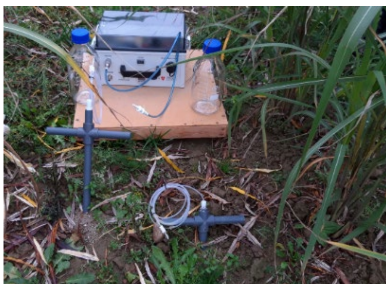
Figure 3.3.7. Lysimeter water sampling in the field experiment.
