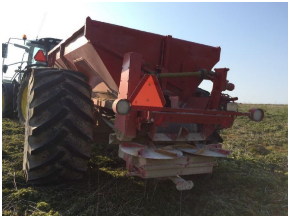
Figure 23. Rear-discharge manure-spreading agricultural equipment. Low rotation on spinning disc to prevent the biochar from spreading too much with the wind
