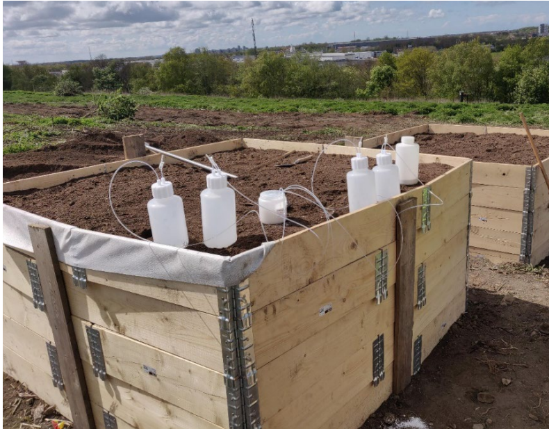
Figure 9. Cultivation beds filled with soil from the landfill top layer and with lysimeters on top, ready to be installed.
