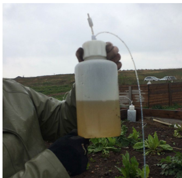
Figure 3.1.5. Lysimeter with soil water from a cultivation bed
