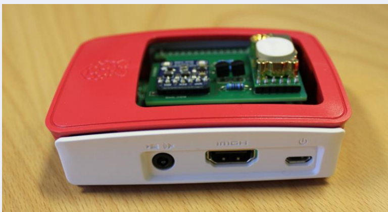
The E.Wattson sensor box measures the temperature, humidity and CO 2 level of the classroom
