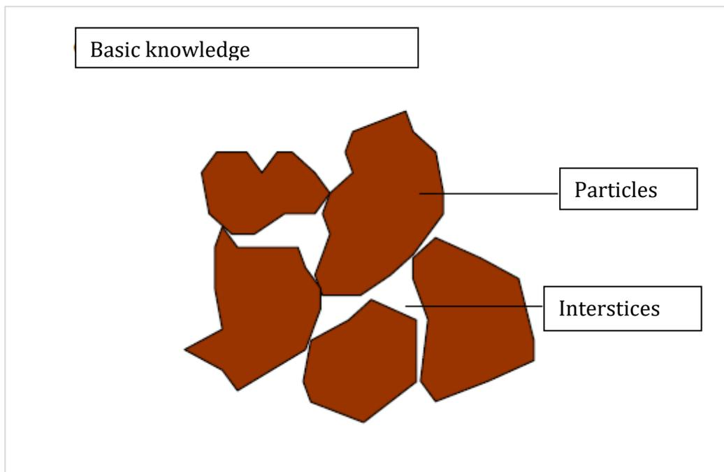
*Picture 6-1: Magnified image of the particles and interstices*
