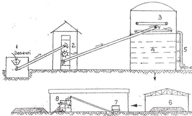
Picture 11-5: Thompson (Carel-Fouché) procedure technological scheme:
