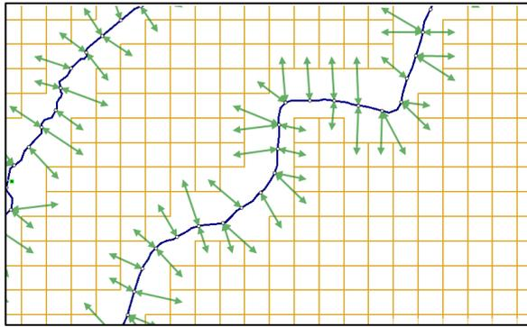
Figure 2.4 Example of a coupled 1D-2D grid.
