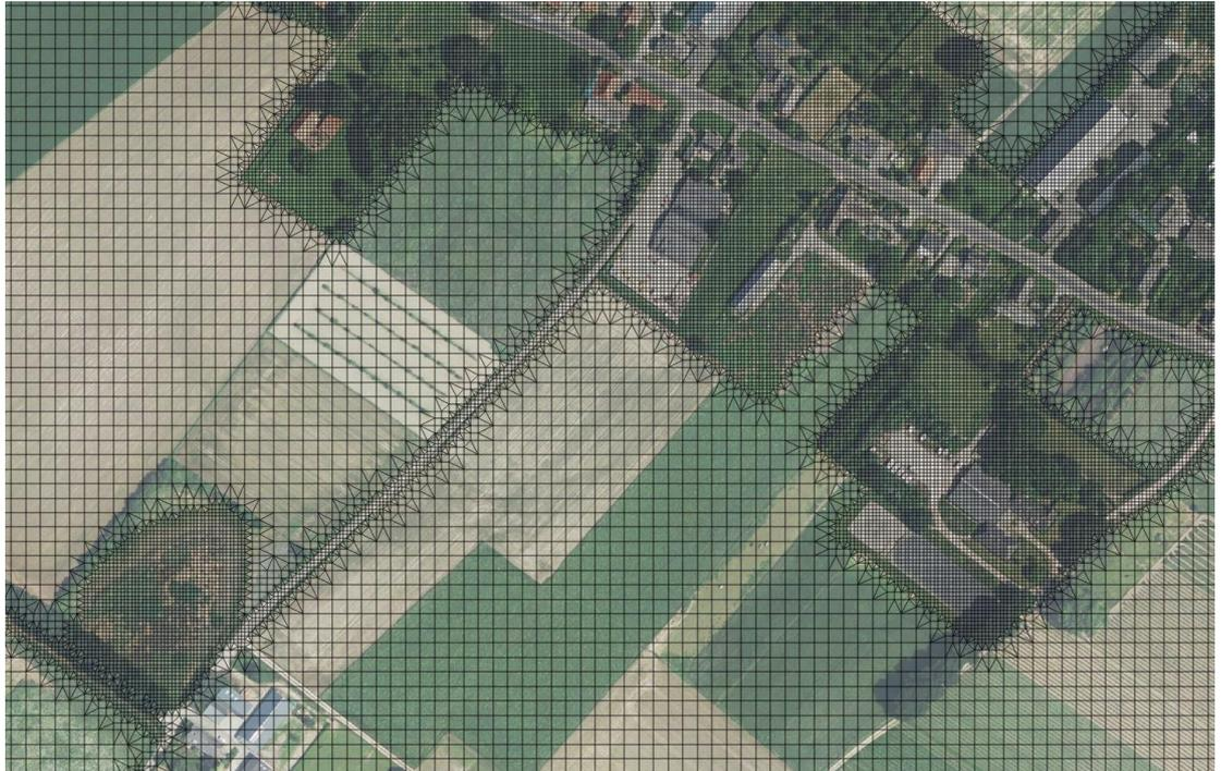
Figure 2.3 Example of a regular grid with local refinements.
