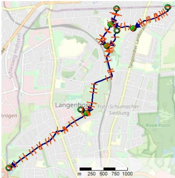
Figure 2.7 Cross-sections (red lines) on the branches of the creeks (blue lines).
