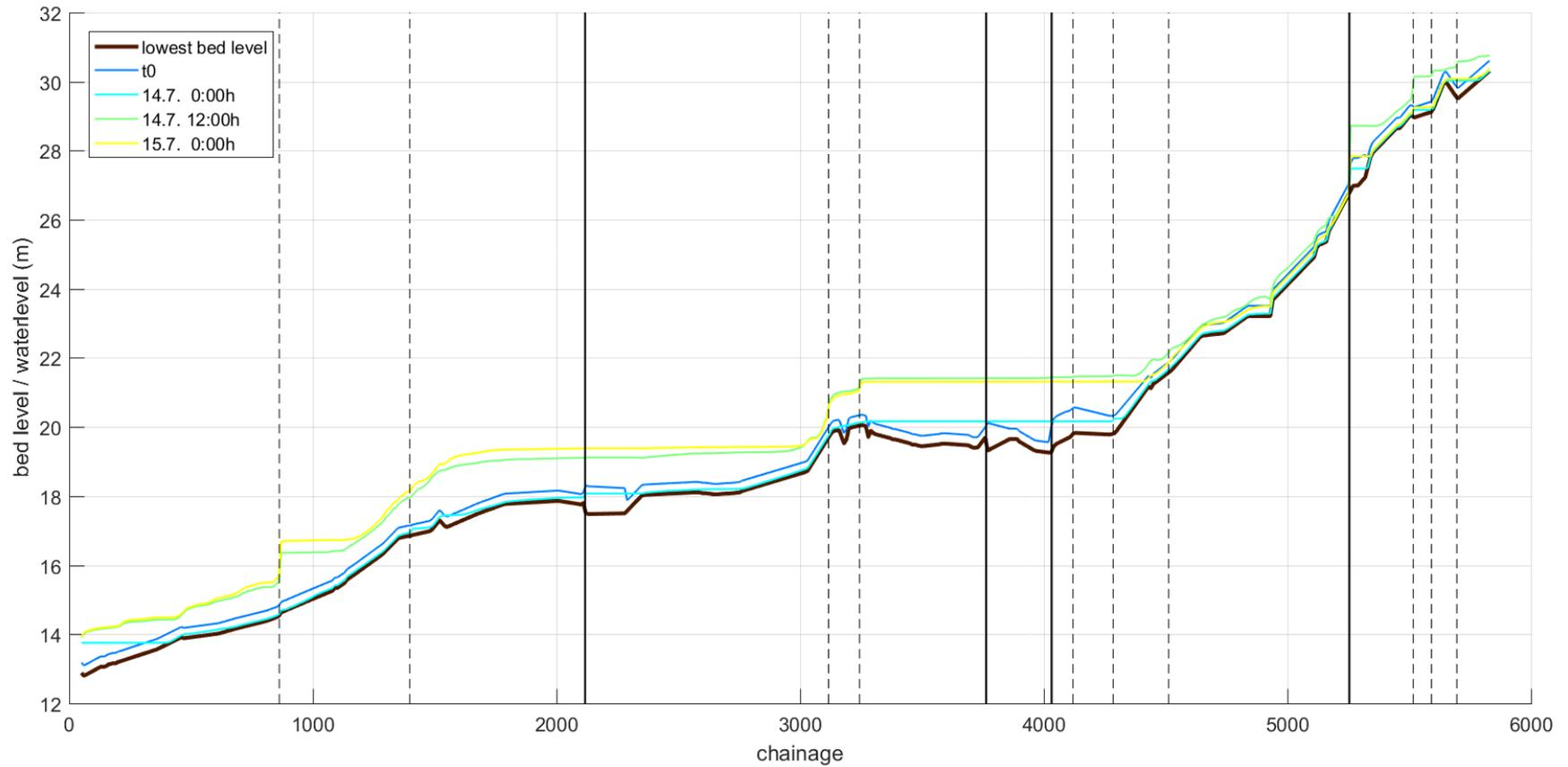
Figure 3.3 Bed level (thick brown line, deepest point) and calculated water levels in Bornbach (1D model).
