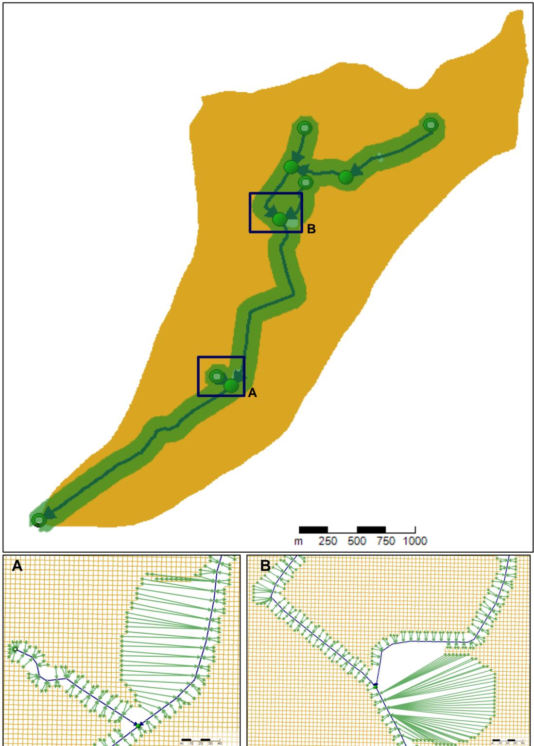
Figure 2.5 Top panel: Full 1D2D grid – blue & green for coverage by 1D, and orange area covered by 2D. Bottom panels: selected details of the coupling at the mouth of Diekmoorgraben and retention basin Diekmoor (A) and the mouth of Tweeltenbek and retention basins Solferinstraße and Kiwittsmoor (B).
