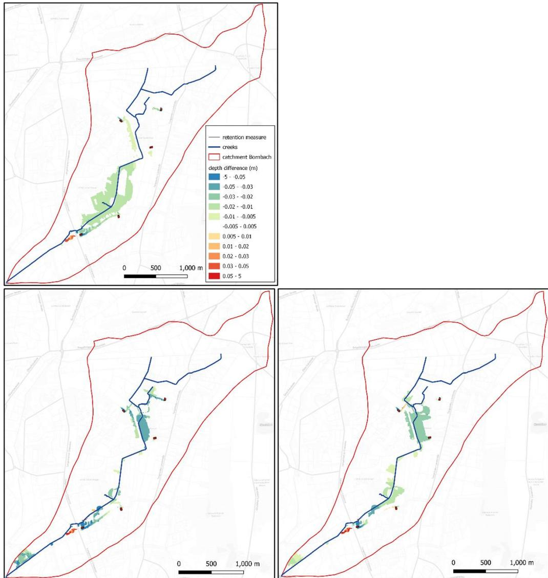
Figure 3.10 Difference in maximum water level (top) and water level difference at 14<sup>th</sup> of July, 5h30 (bottom left) and 8h00 (bottom right).
