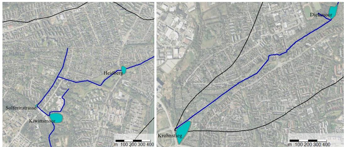
Figure 2.9 Retention (turquoise areas) basins in the Bornbach catchment (black line: catchment delineation, blue lines: creeks).
