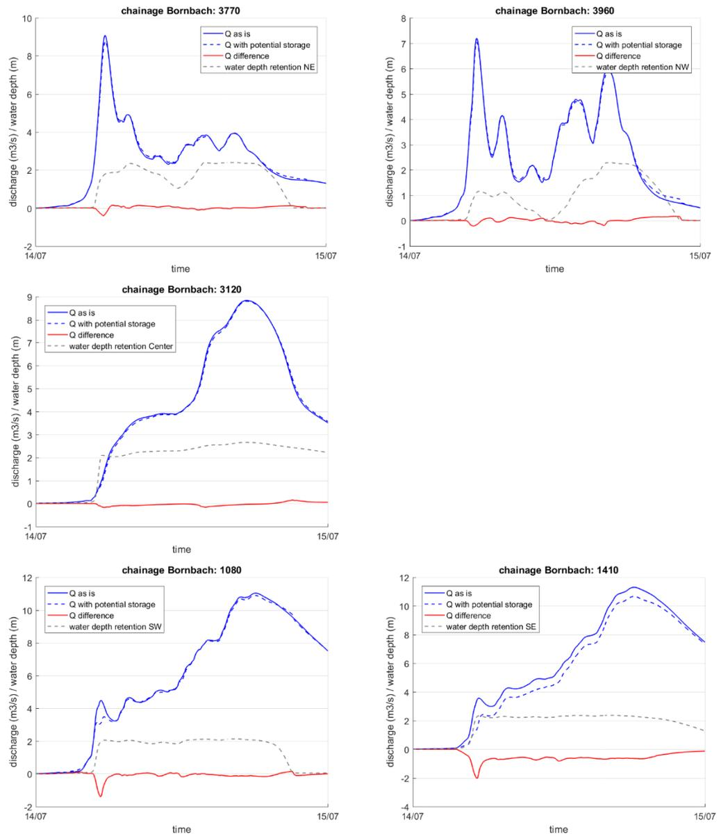
Figure 3.9 Influence on the potential retention measures on discharge in Bornbach creek at selected locations.
