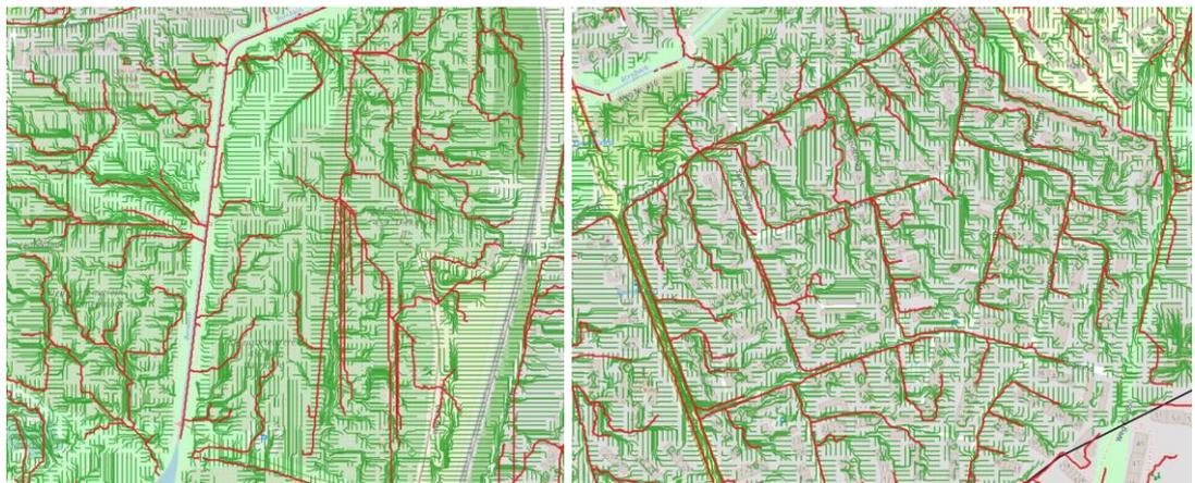
Figure 3.1 Comparison between a GIS flowpath analysis (red) and simulated streamlines (green), with OpenStreetMap as background. Left figure shows the area around Diekmoor, right figure shows the urban area southwest of the Langenhorn Nord station.
