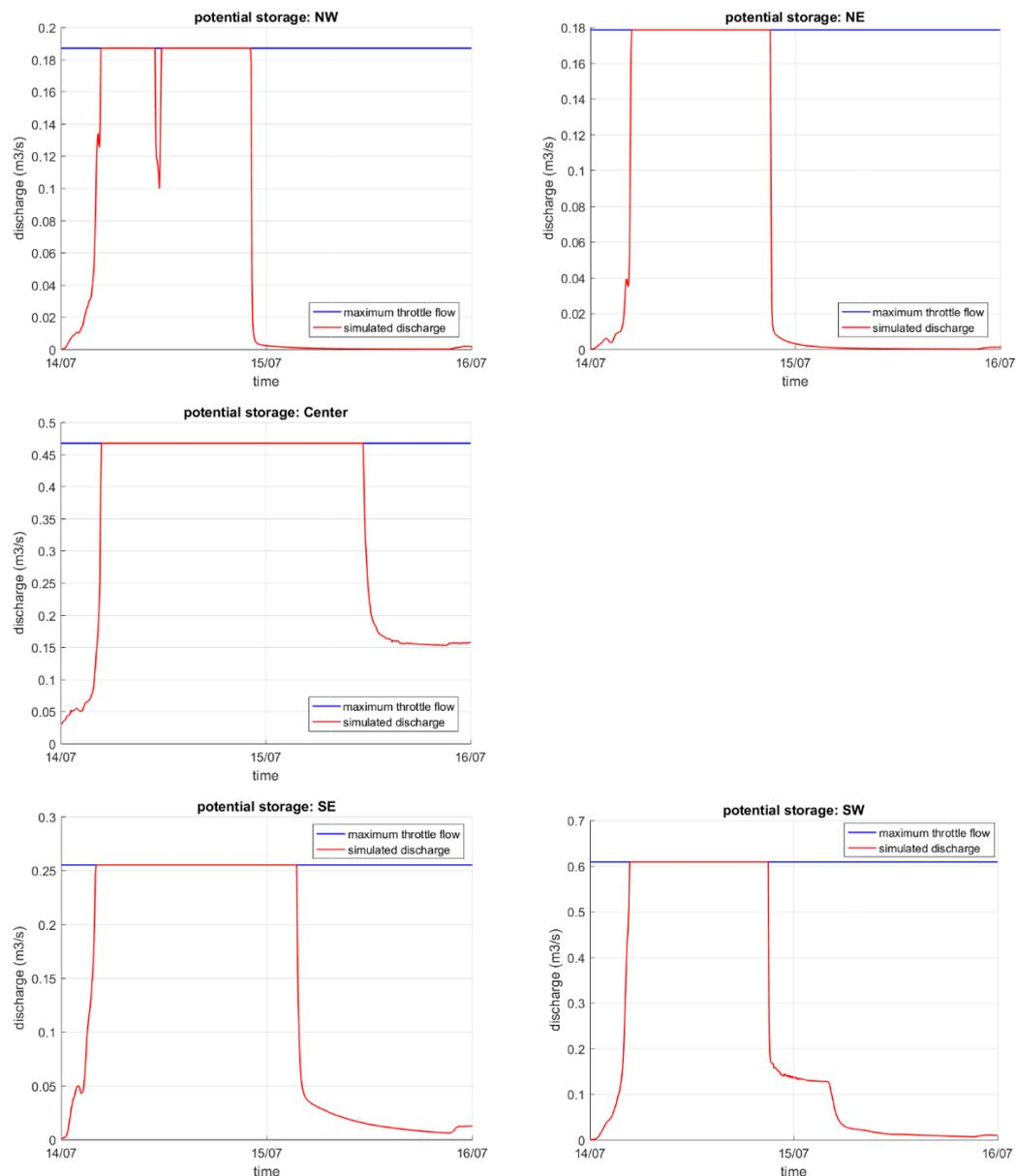
Figure 3.7 Throttle flow out of the potential storage areas.
