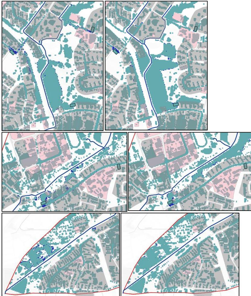
Figure 3.12 Difference in extent of the area with water depth > 5 cm at different locations in the catchment on 14<sup>th</sup> of July, 5h30 (left) and 8h00 (right).
