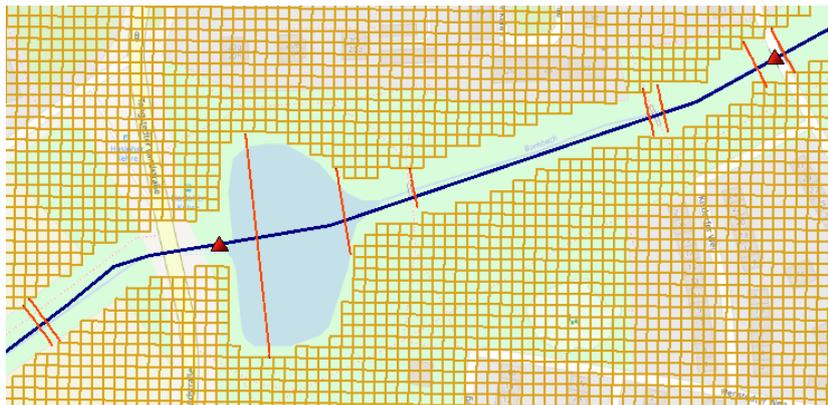
Figure 2.8 Cross-sections (red lines) and hydraulic structures (red triangles) in and around retention basin Heidelberg.
