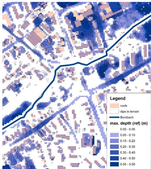
Figure 3.2 Maximum water depth in the catchment compared to the location of dips in the terrain and roofs.
