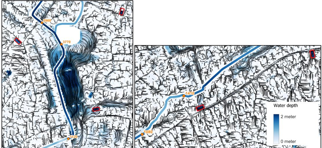
Figure 3.8 Water depth and streamlines (black lines) around the retention measures (red rectangles) on July 14<sup>th</sup>, 15h00.
