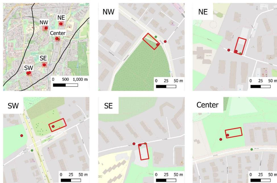
Figure 2.12 Location of the five potential infrastructure measures. Labels in the top left corner indicate the names of the five basins, linked to their relative position within the basin. Green dots indicate the provided locations by LBSG, red rectangles the resulting 20x40m basins, and the red dots the input (within the rectangle) and output (outside the rectangle) location of the added pumps.
