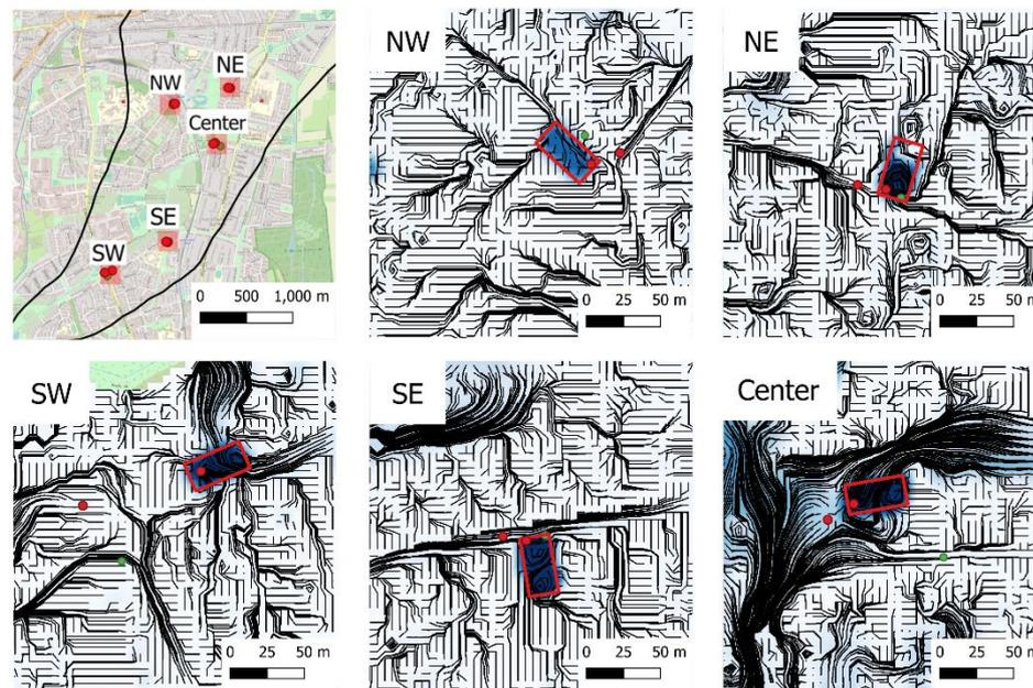
Figure 2.13 Streamlines around the five locations at 2021-07-14 15:00:00. Black lines indicate the flow direction of water at that timestep, coloured background indicates the water depth (white equals to 0 meters, dark blue to +2 meters).
