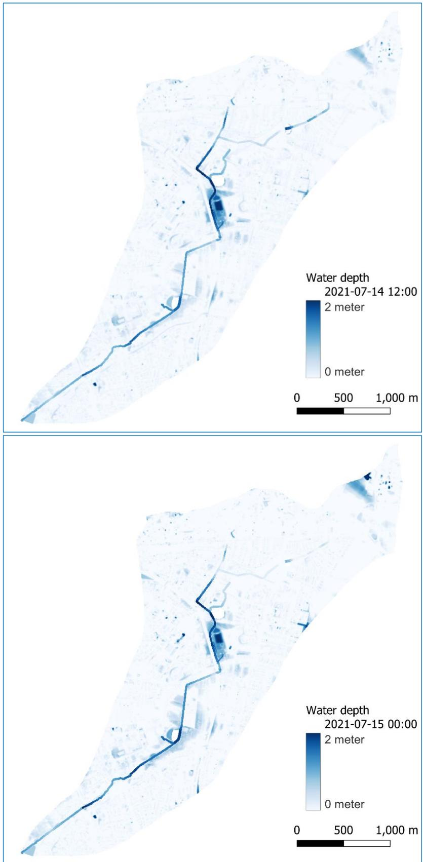
Figure 3.4 Water depths in Bornbach catchment halfway through and at the end of the extreme precipitation event.
