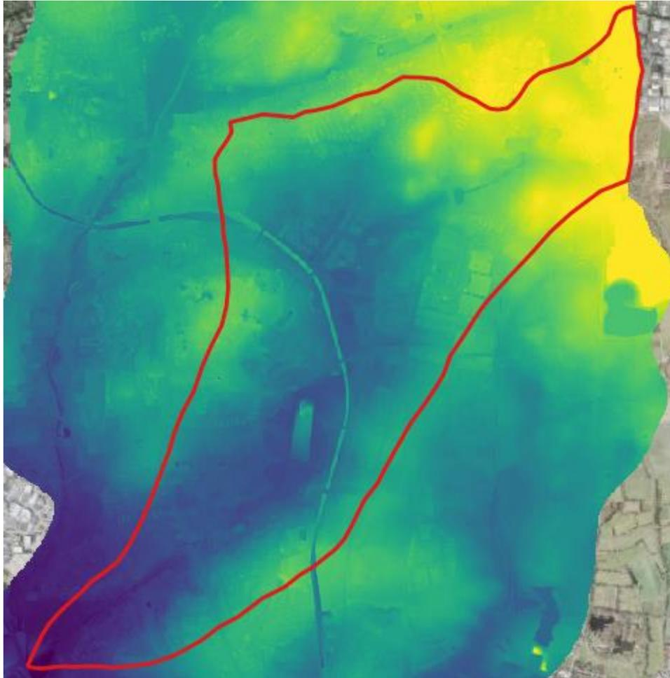
Figure 2.6 Elevation in 1 m by 1 m DEM.
