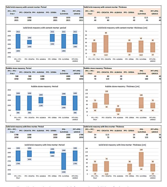
Figure 40 – Comparison between period of construction and thickness for the main masonry types.
