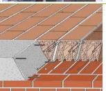
Hollow clay block floor without reinforced concrete slab
