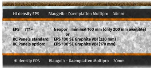
Figure 1. Exterior retrofit insulation system of EPS with 3 exterior cladding of mineral strips
