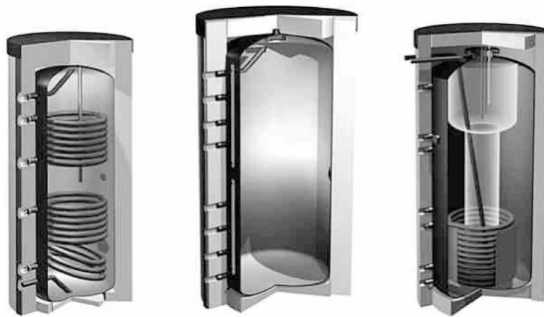
Figure 15: Three different principles of heating storage. Bivalent storage for potable water, buffer tank and a Combined tank with a smaller tank for potable water inside. The coils inside the tanks work like heat exchangers. (Schabbach und Leibbrandt 2014, S. 51)
