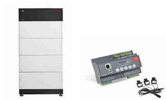
Figure 27: Methods for increasing the own consumption of the solar energy: Storage or direct use. Left: BYD Battery-Box with 5,1 kWh of storage capacity for 3.500 €. Right: Energy manager SMARTFOX Pro - This device switches consumers on and off, if energy is available, so that the own consumption of the generated PV-power is higher. (Cost for this device - 800 Euros) (Voltus.de 2021)
