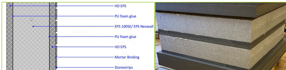
Figure 2.4 - Build up panel & test sample glued EPS (without decoration)
