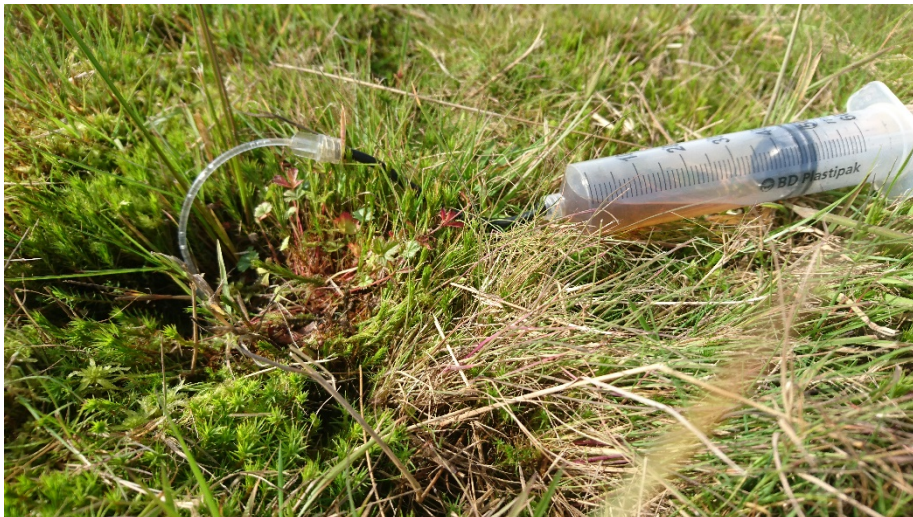
FIGURE 10: SOIL WATER EXTRACTION WITH THE RHIZON
