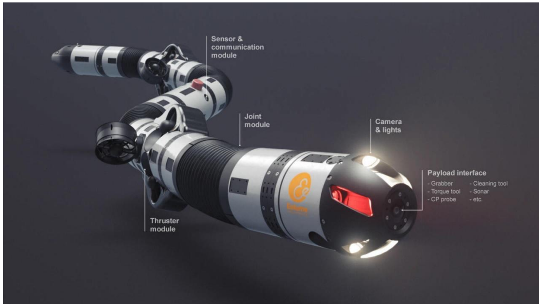
Modular robotic vessel for subsea inspection, maintenance and repair (IMR). Source: Felum
