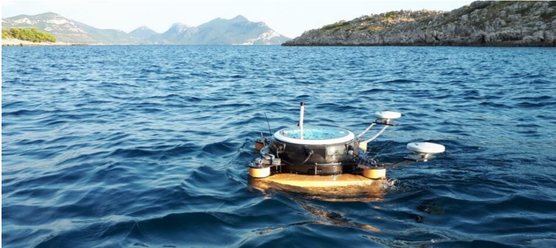
Autonomous USV for water sampling and surface surveying. Source: H2O Robotics
