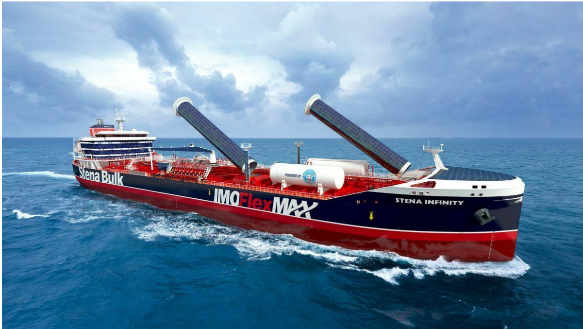
IMOFlexMAX by Stena Bulk, equipped with flettner rotors and solar panels to provide auxiliary power to dual-fuel LNG engine. Source: Stena Bulk
