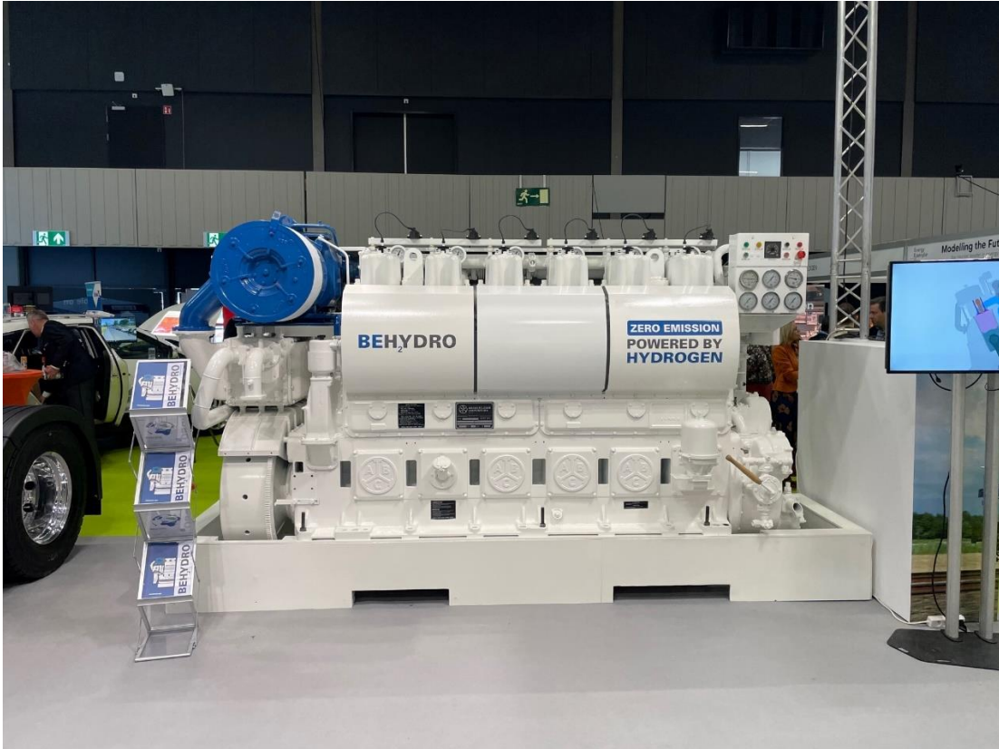
BEH 2 YDRO hydrogen powered spark engine 6DZD model. Source: BEH 2 YDRO
