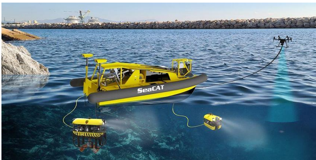
SeaClear's multi-vehicle litter collecting system. Source: SeaClear
