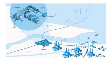
bp's <u>H2Teesside</u> (picture below<sup>21</sup>) is its "world-scale hydrogen project" that would produce 1GW of CCUS-enabled blue hydrogen and start-up in 2027, capturing and sending for storage up to 2mn tonnes of carbon dioxide per year via the Northern Endurance Partnership.
