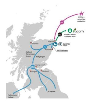
The hydrogen projects involved under the Scottish Cluster include <u>Acorn Hydrogen</u>. Acorn Hydrogen (pictured left<sup>28</sup>) will take North Sea natural gas and reform it to clean burning hydrogen with CO2 emissions created from generation the hydrogen then safely removed and stored using Acorn CCS infrastructure.
