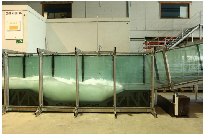
Multifunctional Modular Large Flow Flume at Flanders Hydraulics Research
