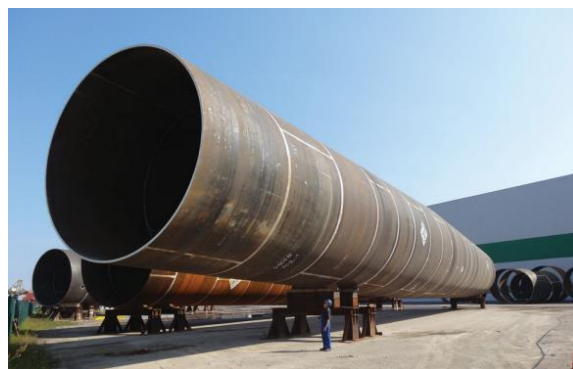
Figure 5 Monopiles for Gode Wind OWF project [66]
