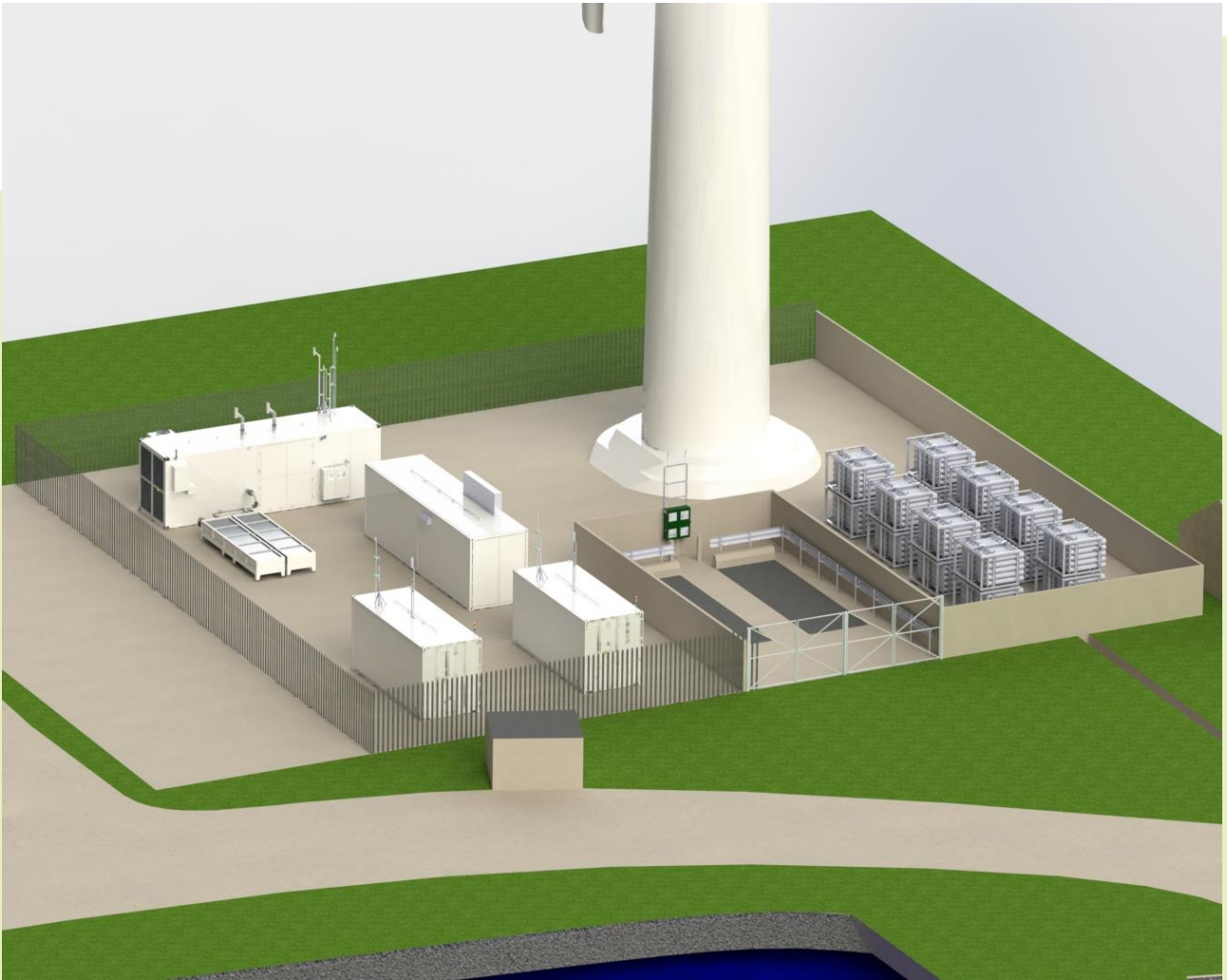
Figure 27 - Close-up view of the electrolyser site, showing the wind turbine, electrolyser, compression equipment, storage vessels and tube trailer connection points.
