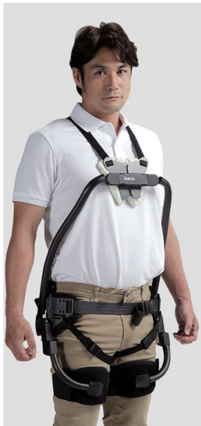
Figure 9. Attachment points between Laevo and wearer.
