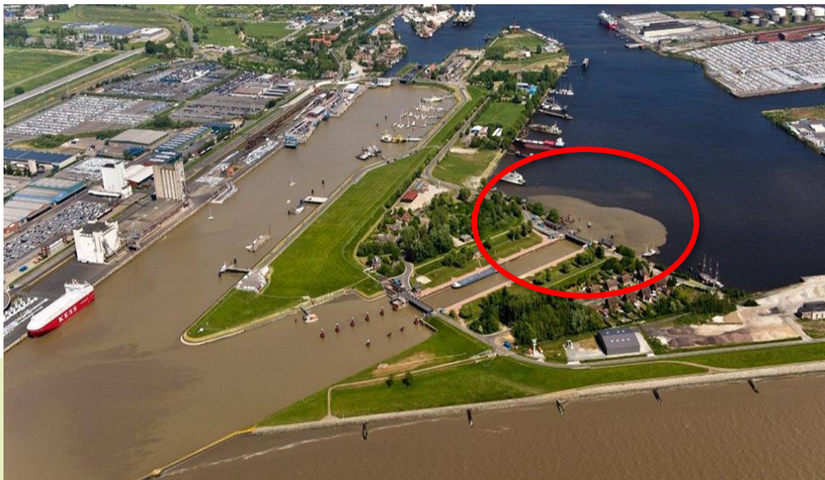
Figure 12. Turbidity difference between the outer and inner port areas and a turbidity plume observed in the inner port.
