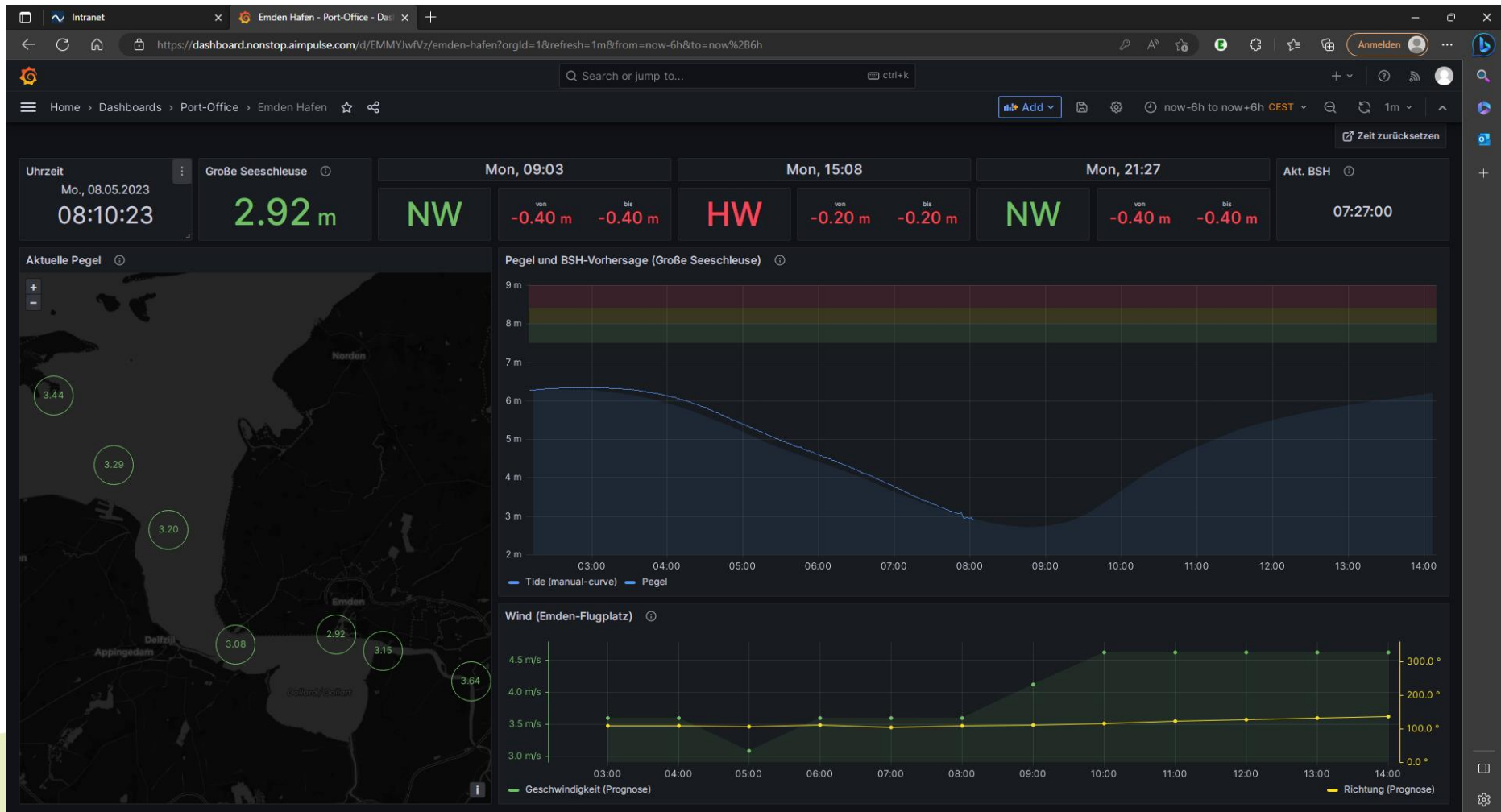
Figure 40. Dashboard created for the Port Office Department, featuring wind conditions, water level measured and predicted values, and customized reference points indicating need for action following a traffic light system.
