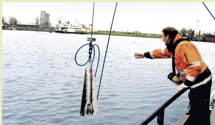
Figure 13. Density measurement being conducted by a crew member on the surveying vessel "MS Delphin" from the Port of Emden. Credits: Synergetik GmbH.
