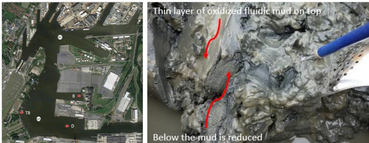
Figure 6. Left: Locations B, TB and D. for sampling of consolidated mud. Right: Example of a consolidated mud sample.
