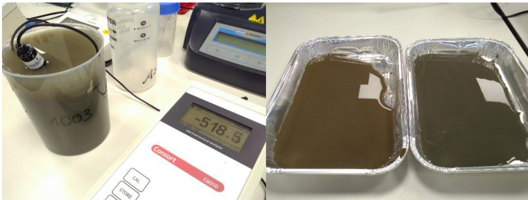
Figure 3. Examples of direct measurements of fluid mud properties. Left: Redox potential of sample 1003 (IH). Right: Visual observation of fluid mud samples. Brownish discoloration is typical for more oxidized fluid mud from GS (sample 1001) and grey colours indicate more reduced oxygen in fluid mud from IH (sample 1003).
