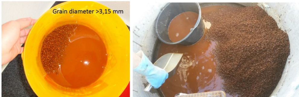
Figure 11 Sieved and rinsed ICS as P filter material. The grain size is >3.15 mm in order to achieve a sufficient saturated hydraulic conductivity with a prevailing low hydraulic gradient in the field.
