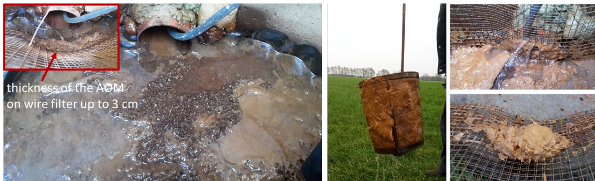
Figure 5 Input of amorphous organic matter (AOM) from the drainage pipes into the individual filter stages of the experimental inline P filter.
