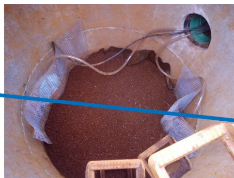
Figure 10 Pre Filter (left) and P Filter (right), the blue arrow indicates the flow direction. Transparent hoses: suction of the drainage water samples in the inlet and outlet, dark cable: flow measurement upstream of the P filter in the drainage pipe.
