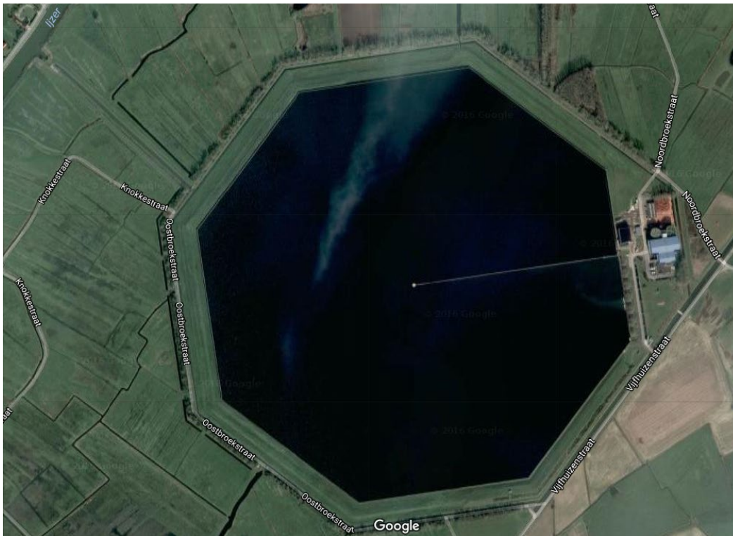
Figure 1 De Blankaart water reservoir covering a surface area of 63 ha with a volume of 5.670.000 m 3
