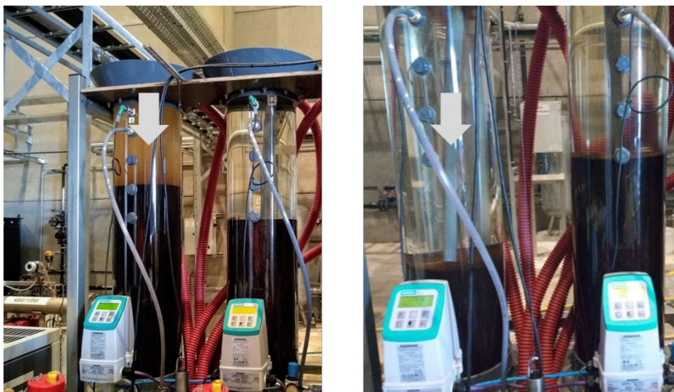
Figure 4 The column filled with the ABA-100 material, immediately after bringing it in contact with the influent (left), and the same column after 4 hours of treatment at a flow rate of 200 L h -1 (right). In both pictures, the right column is filled with a stable material, which can serve as a reference for the height of the ABA-100 material in the left column.
