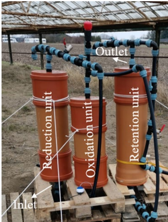
Fig. 2: Photo of the ZVI filter system field experiment
