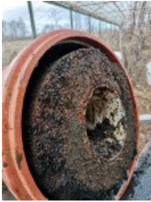
Fig. 8 – Corroded ZVI material stained brownish-red by the ochreous material at the inlet of the ZVI filter
