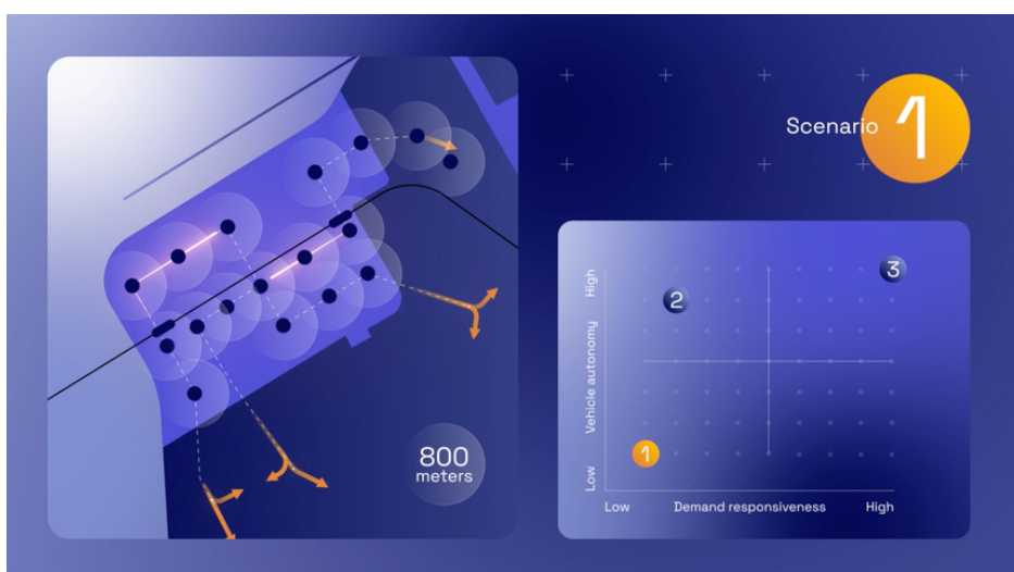
Figure 2: Diagram of public transport scenario 1 in Almere, depicting two fixed BRT lines with independent stops 800m apart.
