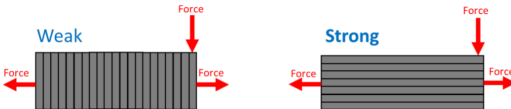
Figure 15. Schematic showing strength knockdown perpendicular to the layers.
