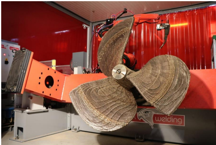
Figure 32. A ship propeller formed from WAAM.
