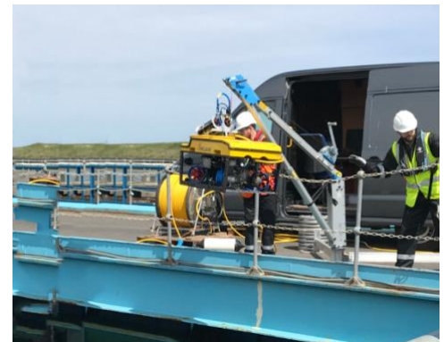
Figure 31 Rovco's 3D visualisation system in testing at the Catapult's National Renewable Energy Centre in Blyth.
