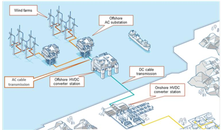
Figure 18 Diagram showing the transmission system from wind farms to landfall point via various cables, substations and converter stations. (Source: ABB)
