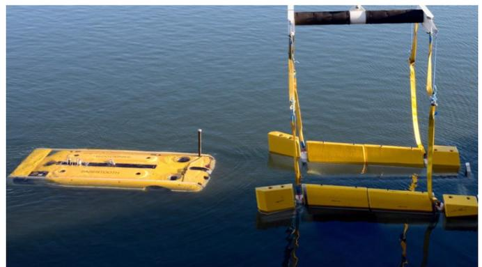
Figure 20 Modus and Osbit. AUV and docking station
