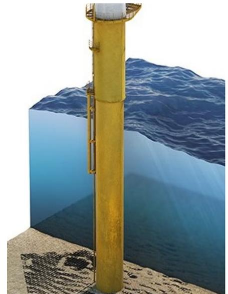
Figure 16 Fixed Offshore wind turbine foundation
