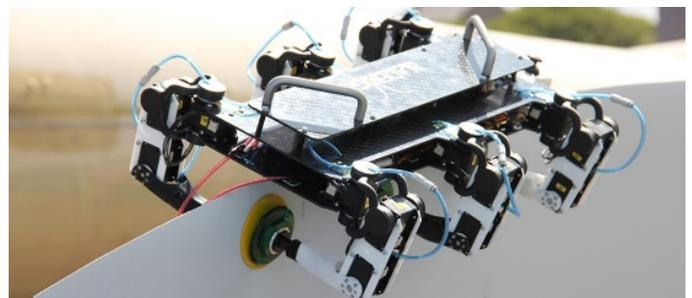
Figure 22 Blade Bug. Wind turbine blade repairs
