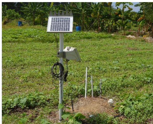
Figure 19: Soil sensors that measure salinity levels on Mahé (CBA, 2016).
