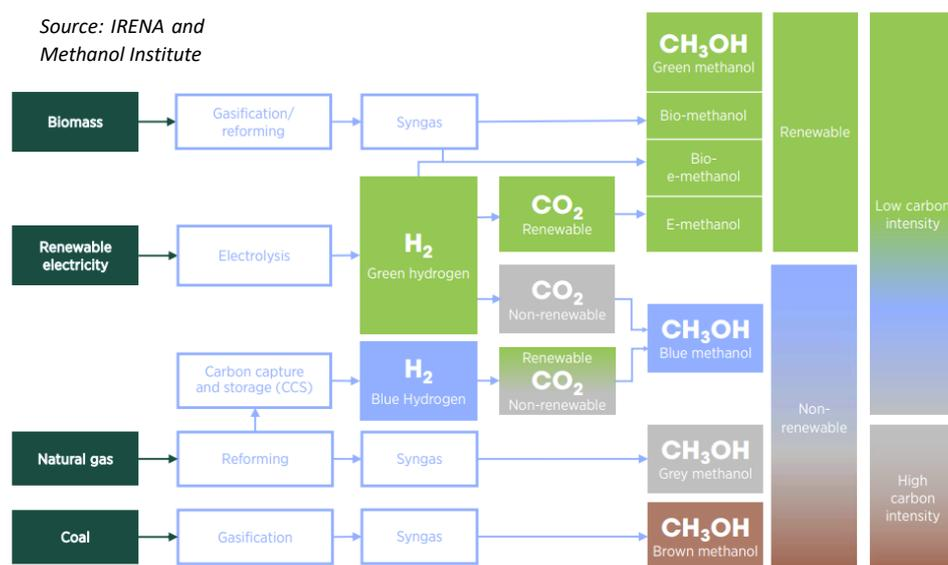
Figure 4: Different methanol production pathways
