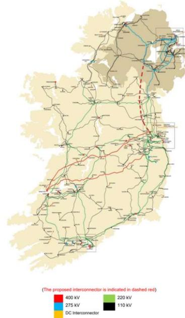
Figure 2: Map Showing Transmission Network and Proposed Interconnector<sup>36</sup>
