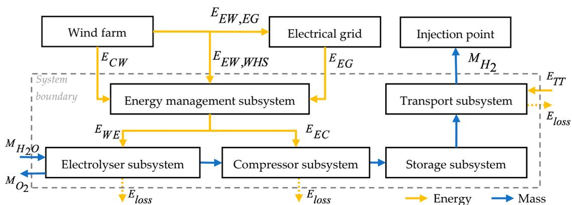
**Figure 1.** Block diagram of a wind-hydrogen system (WHS) which is located at each wind farm in Ireland.
