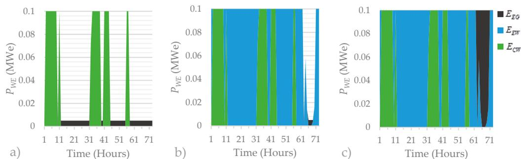
**Figure 2.** Scenarios of electrolyser operation mode: (a) curtailed wind operation, (b) available wind operation, and (c) full capacity operation.
