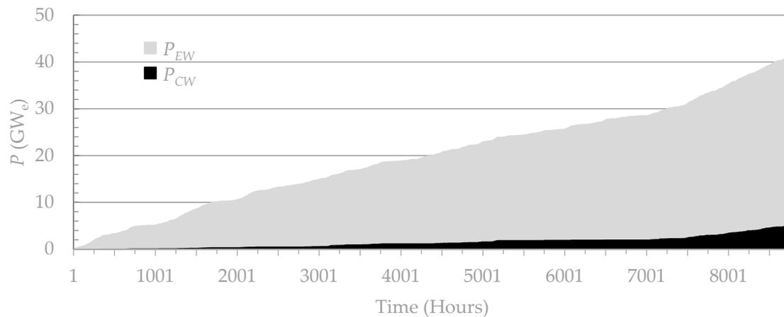
Figure 5. Cumulative wind power profile of a sample wind farm.
