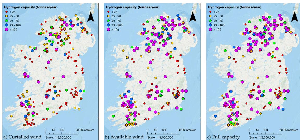
**Figure 8.** Capacity of annual hydrogen production ( $M_{H_2}$ ) with current parameters of (a) curtailed wind operation, (b) available wind operation, and (c) full capacity operation, calculated by the techno-economic submodel for all wind farms in the island of Ireland.
