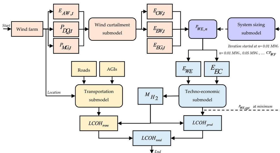
Figure 4. Algorithm to calculate the  $LCOH_{total}$ .
