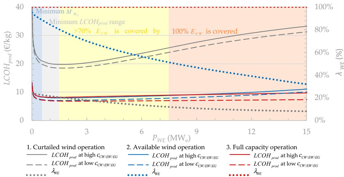
**Figure 6.** Calculated  $LCOH_{prod}$  for Ballincollig Hill wind farm as a function of electrolyser size for all operation scenarios.
