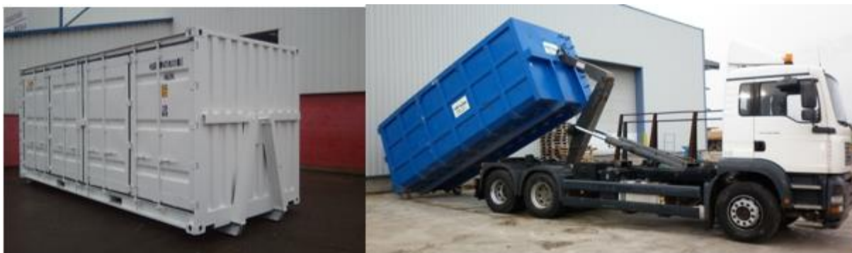
Figure 1 – 20' ISO ampliroll compaction container for the transfer of residual household waste (OMR)
