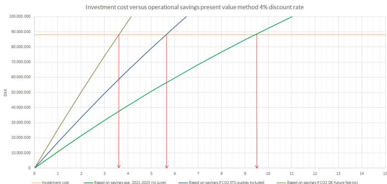
Figure 5.3.2 Accumulated savings discounted to present value with discount rate of 4% versus present investment cost incl. VAT of 16% for shore-based charging stations and profits from grid balancing FCR services. Source EMK.
