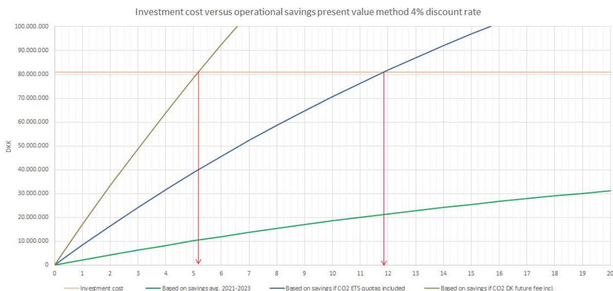
Figure 5.1.1 Accumulated savings discounted to present value with discount rate of 4% versus present investment cost incl. VAT of 16% for shore-based charging stations. Source EMK.
