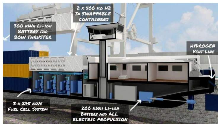
Figure 1 : Side cutaway illustration of H2 Barge 1 Hydrogen system
