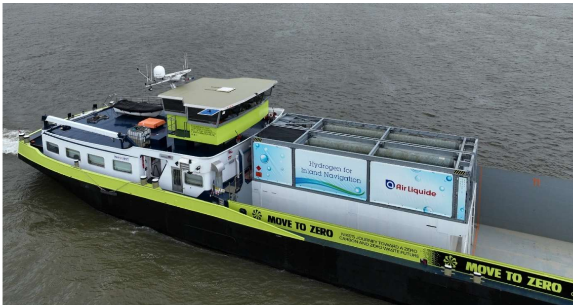
Figure 1. H2 Barge 1 (formerly the FPS Maas) sailing on Green H2.
