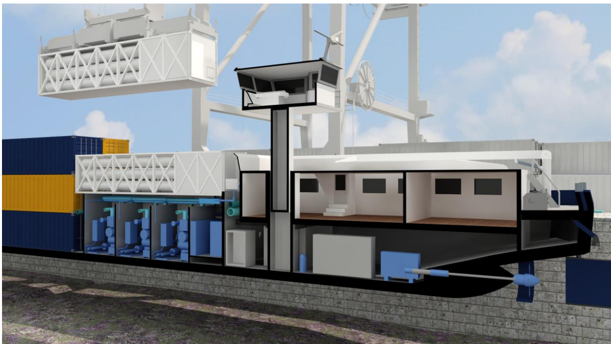
Figure 2. The Maas will be retrofitted with PEM fuel cells and hydrogen fuel storage.
