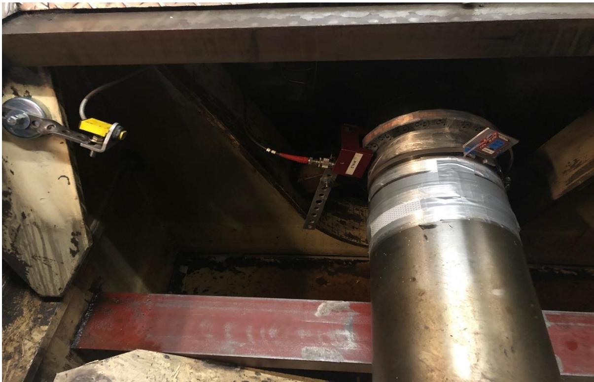
Figure 3: Measuring set up on the main shaft with rpm sensors and strain gauges.
