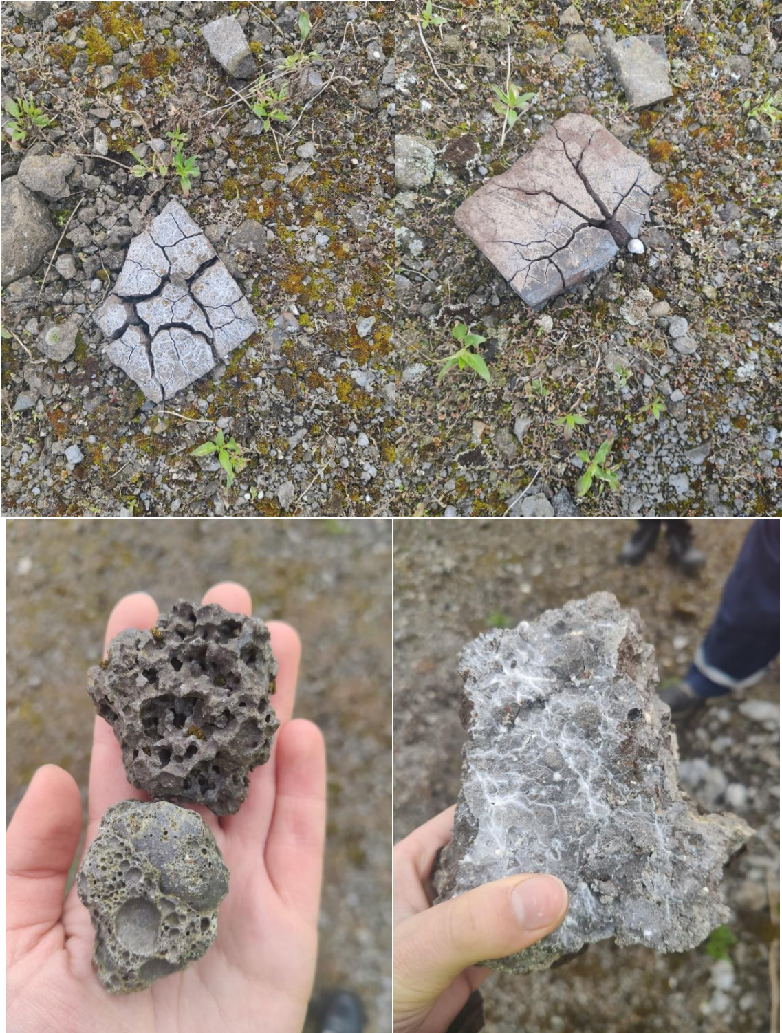
Figure 10: Range of slag characteristics observed on site: weathering type, porosity and veining
