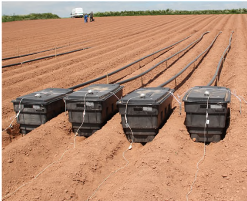
Figure 7. A typical runoff and erosion plot layout.
