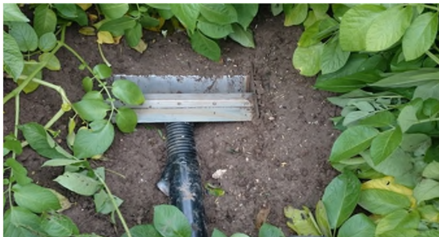
Figure 9. Gerlach trough bedded into the wheeling to capture runoff from within the 30m plot.
