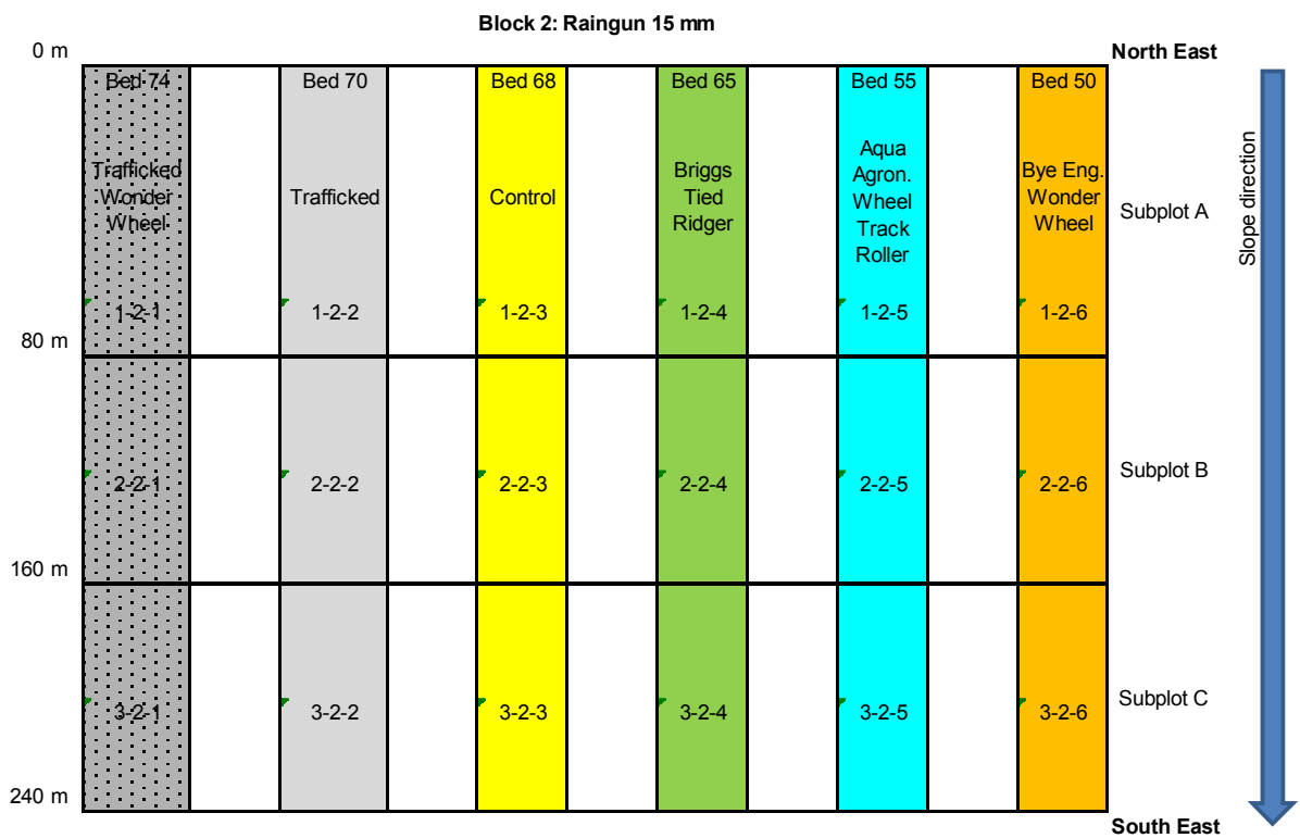
Figure 6. Treatment layout and subplots within each experimental block.
