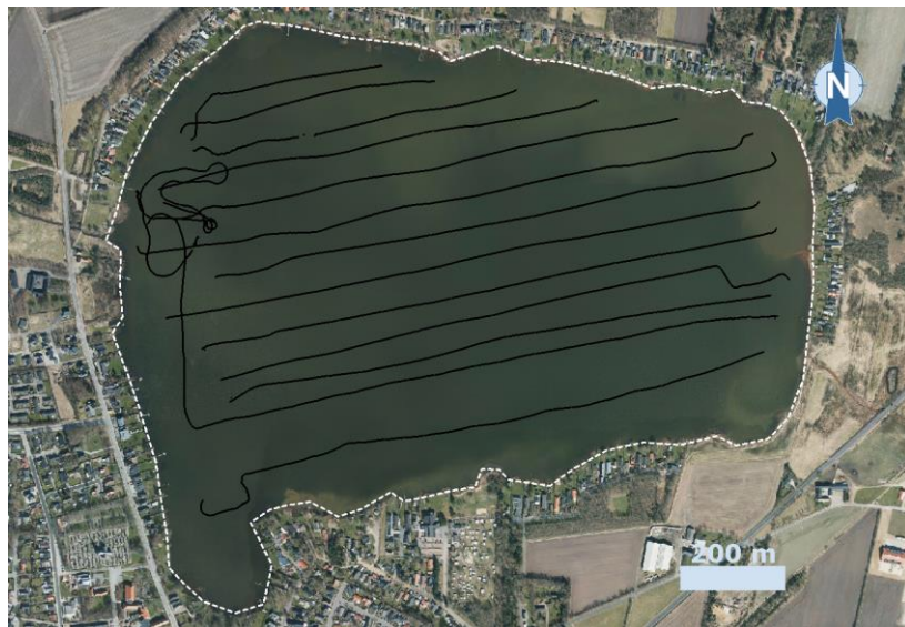
Figure 1. Survey area, with FloaTEM lines in black. Each black dot corresponds to one FloaTEM sounding. The line spacing is ~60 m.
