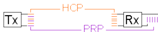
Figure 1. Sketch of the transmitter (Tx) and receiver (Rx) coils in a DUALEM-421S system. For the HCP-configuration the Rx-coil is placed on the same horizontal plane as the transmitter coil. For the PRP-configuration the Rx-coil is perpendicular to the Tx-coil and centered around the Tx-coil's horizontal plane.
