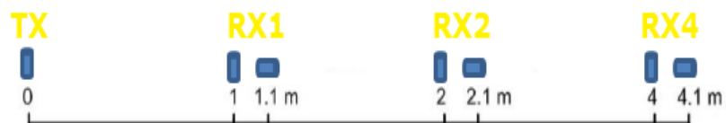
Figure 2. Sketch of the DUALEM-421S instrument. The transmitter coil (Tx) is placed at one end of the tube and the 3 receiver coil pairs (Rx) at a distance of 1, 2, and 4 m from the transmitter coil.
