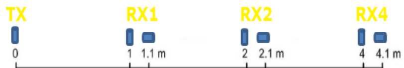
Figure 2. Sketch of the DUALEM-421s instrument. The transmitter coil (Tx) is placed at one end of the tube and the 3 receiver coil pairs (Rx) at a distance of 1, 2, and 4 m from the transmitter coil.
