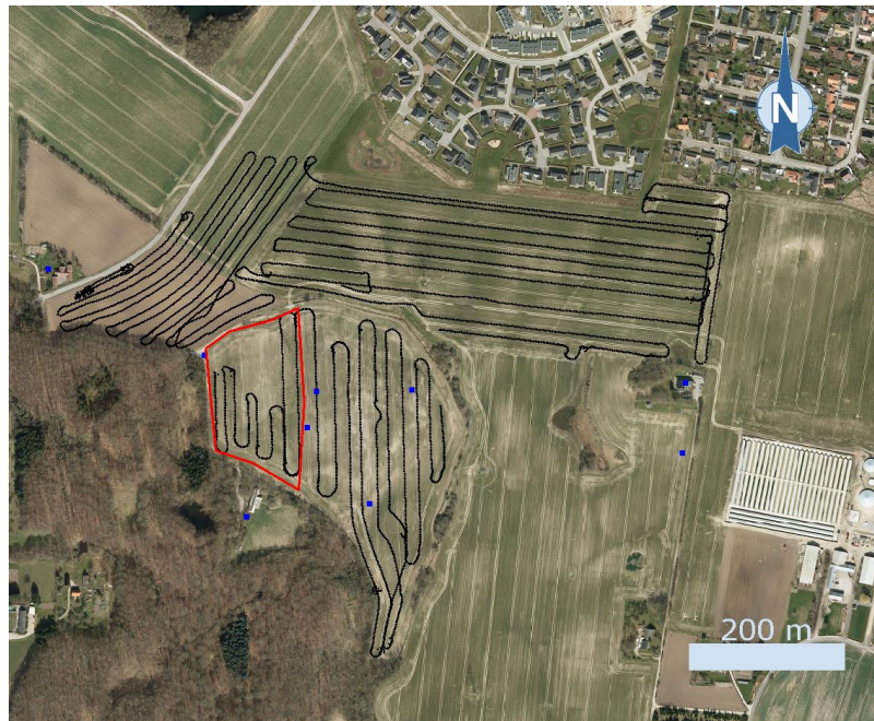
Figure 1. Survey area, with tTEM lines in black. Each black dot corresponds to one tTEM sounding/resistivity model. The model spacing along the lines is ~10 m. The blue circles shows boreholes in the area.
