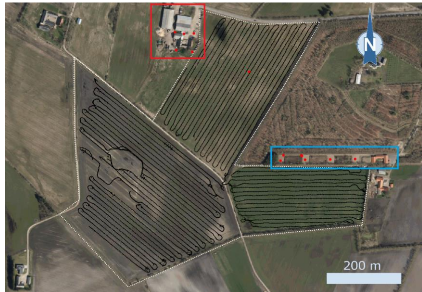
Figure 1. Survey area, with tTEM lines in black. Each black dot corresponds to one tTEM sounding/resistivity model. The model spacing along the lines is ~10 m. The red circles shows boreholes in the area.
