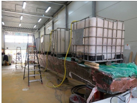
Fig. 15: Impression of the load test using seven water tanks
