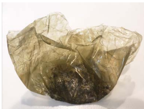
Figure 2. A sample of PHA film produced directly after the solvent recovery. The dark green color was common to all of the samples produced.
