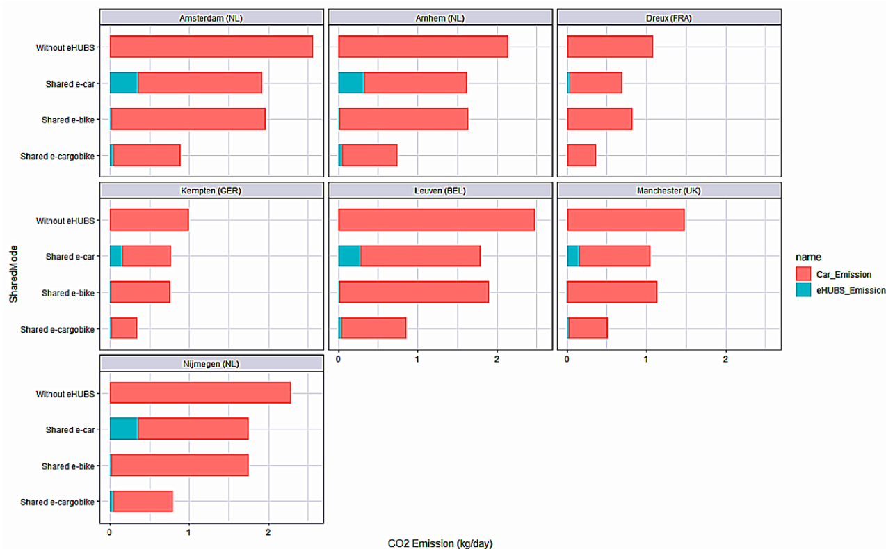
Figure 17. Shared mobility users' emissions without eHUBS and with different modes of eHUBS of all cities.
